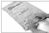
2- Alternately "pat" back and forth on the "A" and "B" ovals fifteen to twenty times. As soon as the foam begins to expand, place the bag into the empty case. NOTE: Instapack foam expands rapidly so work quickly.
