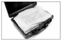
4A- Activate a second bag. Quickly place on top of the product. Close the case lid and lock for 30 seconds so that the foam expands to form a top cushion.
