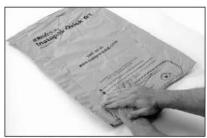
1- Completely unfold an Instapack Quick® RT bag and lay on a flat surface. Press hard on the component "A" oval to break the seal.
