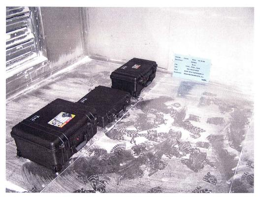
Photograph 1 Dust Test Setup (Tested with other Pelican Product Items)
