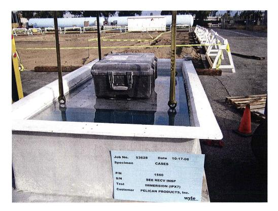
Photograph 4 Immersion Test Setup
